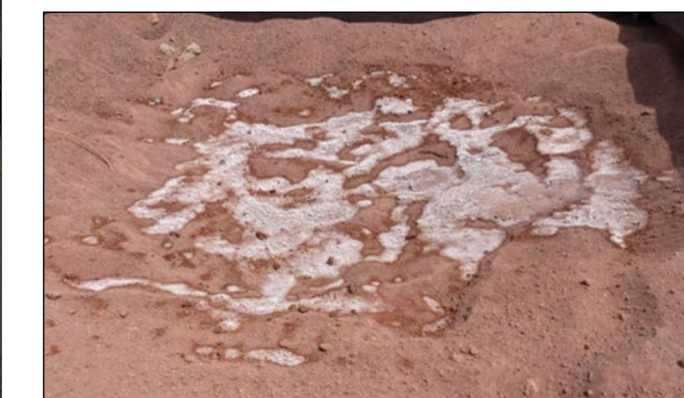
Simulated cemented icy regolith
