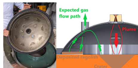
Figure 4: Dome interior (left) and illustration of expected gas flow path during testing (right)
