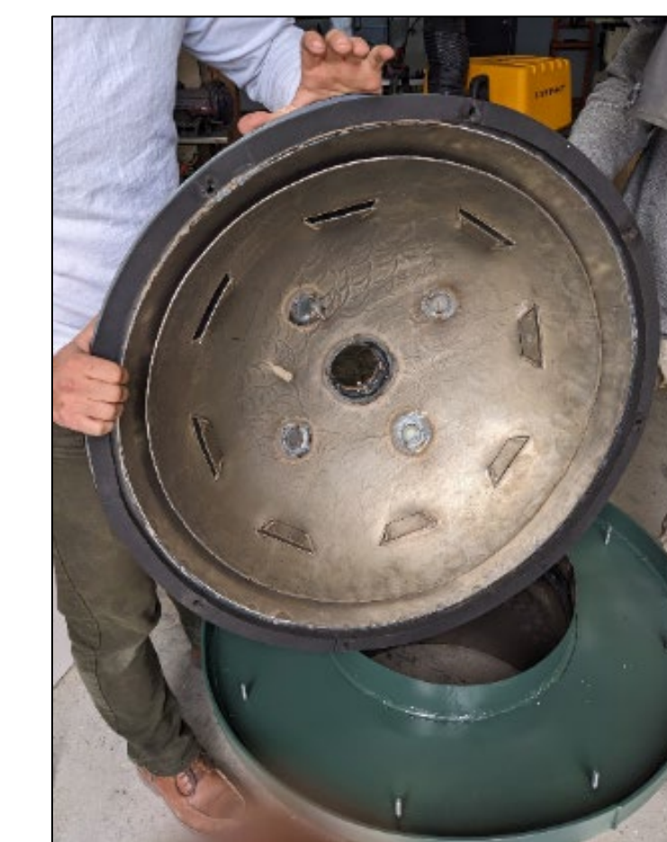
Fabricated dome; Removeable top for inspection between test fires
