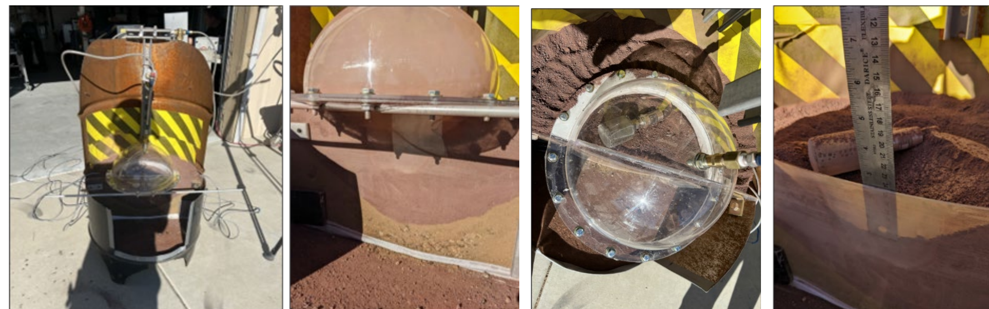
Cold gas test setup with nitrogen gas nozzle, dome prototype, split view window, and post-test measurement
