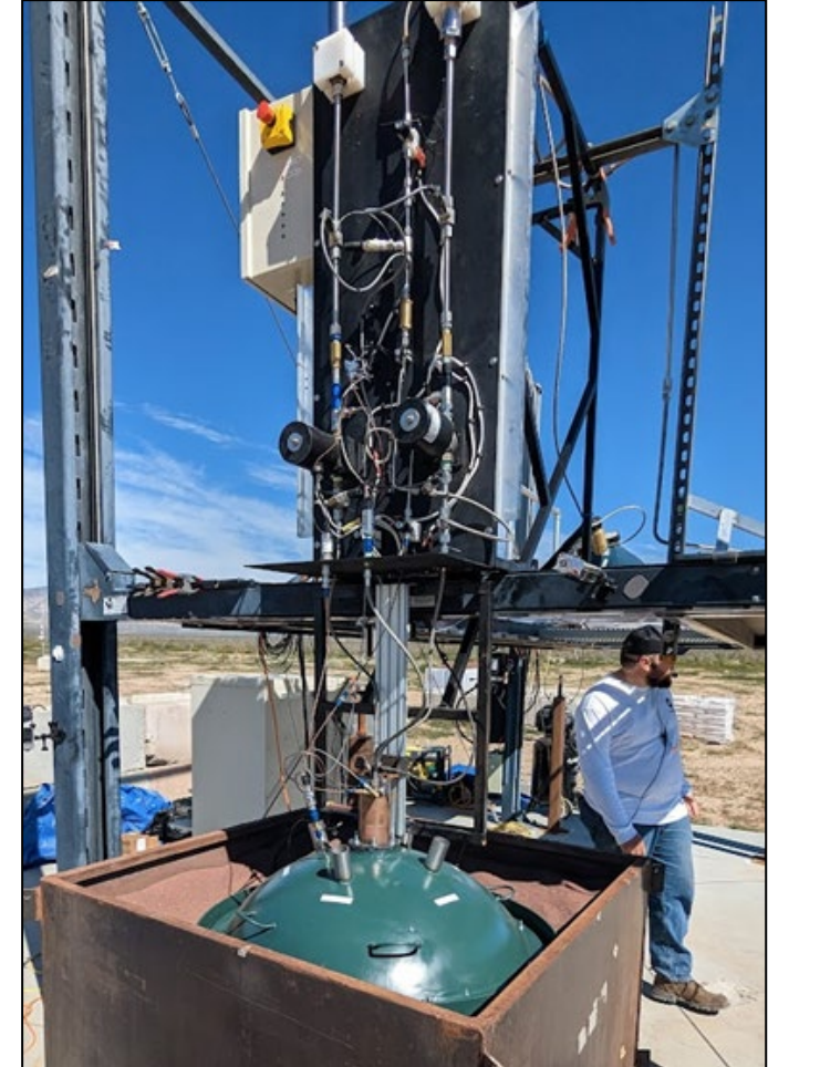
Dome integrated with rocket test stand
