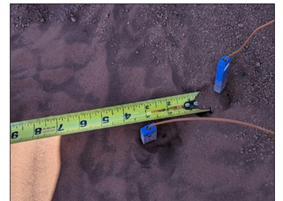
Thermocouples placed to detect thermal transfer into regolith adjacent to crater
