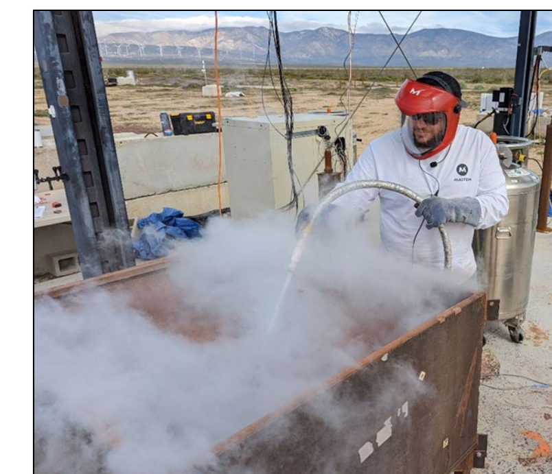
Prepping icy regolith with liquid nitrogen
