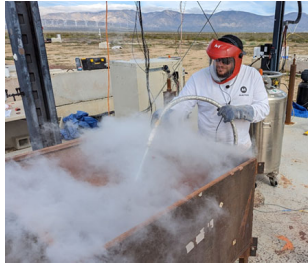
Figure 6: Chilling icy regolith with liquid nitrogen
