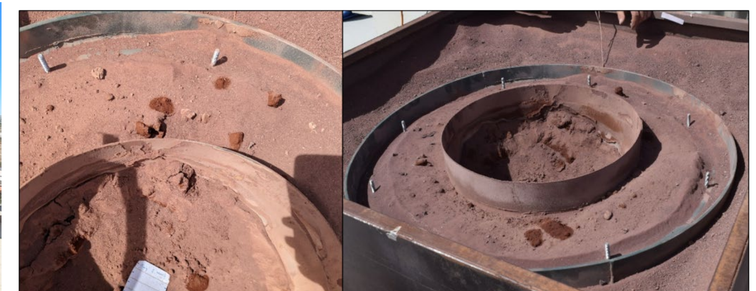
Melted ice observed in collection tray after hot fire; The team theorized that ice crystals were likely collected, but then melted due to sitting in 80° F ambient conditions before observations could be made after each test
