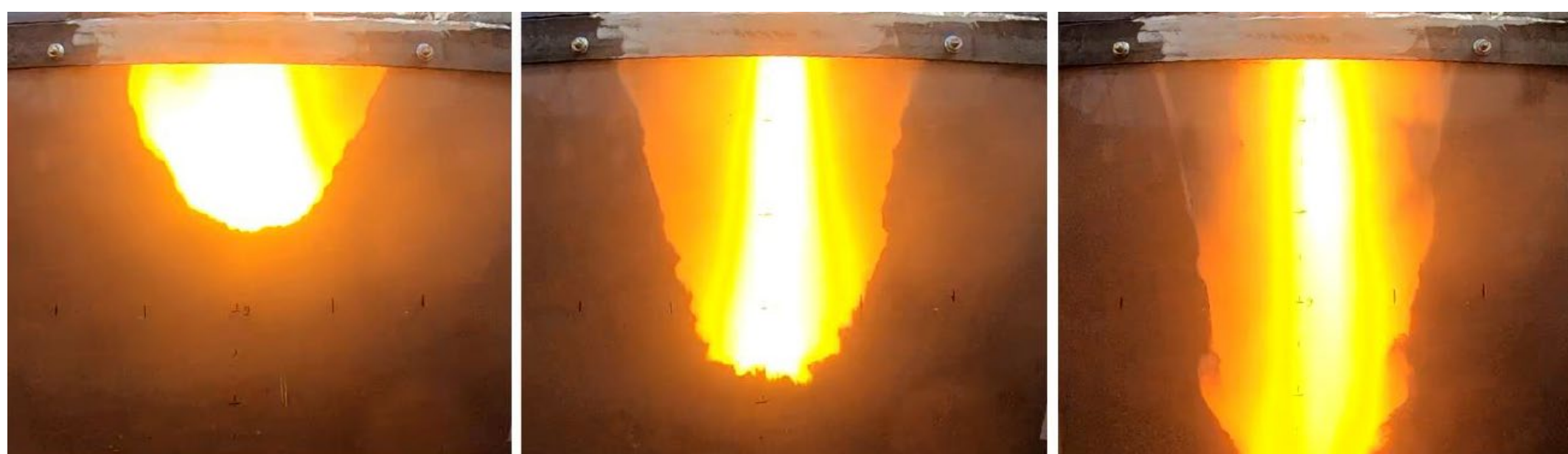
Regolith deep cratering demonstrated during plume-surface interaction testing
